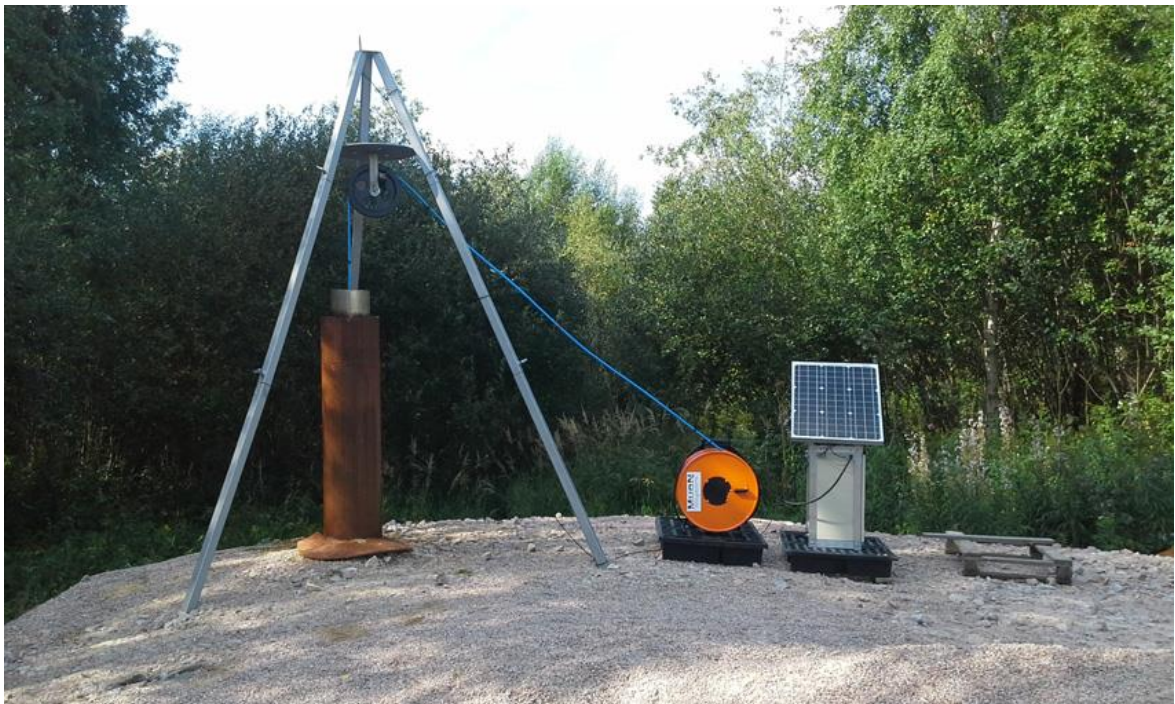
Fig. 1. A borehole muon detector in action in a groundwater production well in Kurikka, Finland. This particular muon monitoring system is equipped with solar panels and external modem antenna for remote control and data transferring purposes. Figure courtesy by Muon Solutions Oy.
