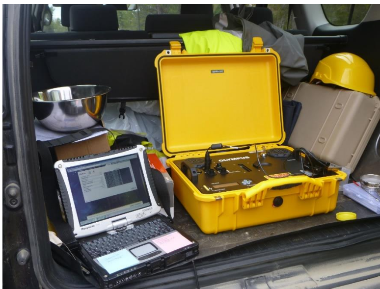
Fig. 1 Olympus Terra pXRD analyzer in field use
