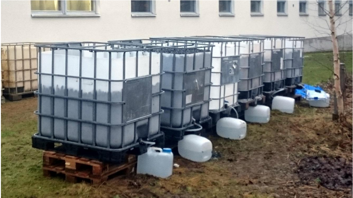
Fig. 1. Filled in lysimeters to study leaching behaviour of waste rocks in varying conditions. Photo © Teemu Karlsson, GTK.
