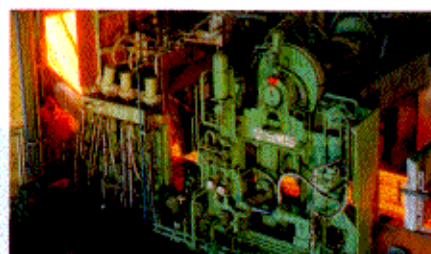
CSP - the leading thin-slab casting and rolling process for the production of high-grade hot strip.
