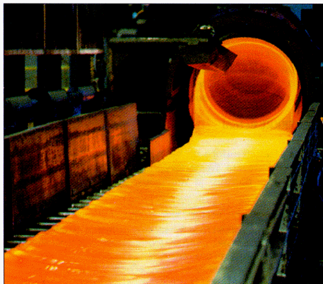
Figure 2. Wire rods are coiled after hot rolling at Fundia Wire in Dalsbruk.
