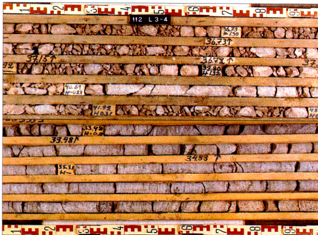
Fig 3. Hazardous weathered rock-gouge drilled for siting the Päijänne tunnel. Lower box represents moderately fractured solid bedrock.
