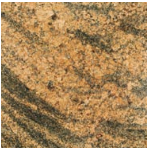
Figure 1. Image of a 30x30 cm rock plate obtained by using a CCD-digital camera.
