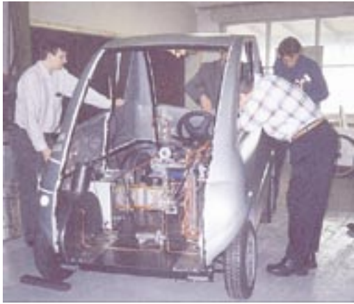
Figure 9. Finnish commercial AFC with hydrogen storage and AFC pack installation into a "Fantasia" fuel cell car prototype (source: Hydrocell Oy).
