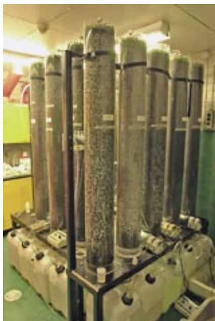
Figure 5. Column bioleaching tests with 60 kg of ore.
