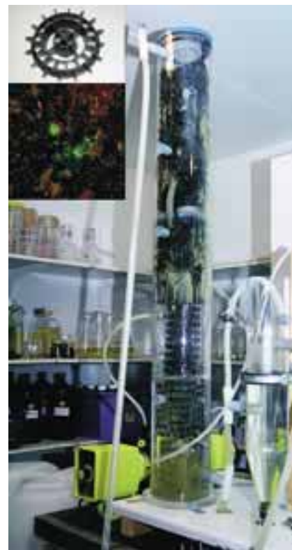
Figure 3. Biofilm-reactor with carrier disk and micrograph of the biofilm (photos by Jouni Hyvärinen/Meila and Katri Mattila).
