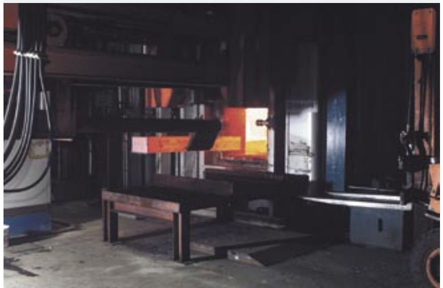
MEFOS's 3 tonnes/hr walking beam furnace which was used for tests of flameless oxyfuel combustion technology (photo: Michael Törnkvist, LuleBild).
