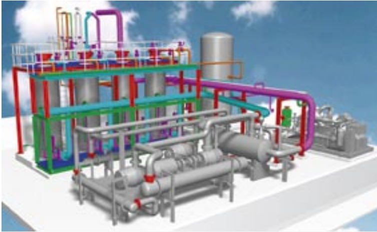
View of VPSA unit in Luleå (picture Air Liquide).
