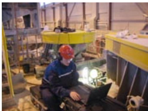
McGill Bubble Size Analyser being operated by researcher Tatu Miettinen (photo courtesy of Kemira GrowHow, concen- trator Siilinjärvi).
