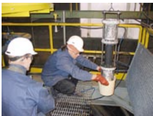
Researcher Rodrigo Grau operating the air hold-up probe. Hold-up is the volumetric fraction of air in the air-slurry phase (photo courtesy of Boliden Harjavalta).
