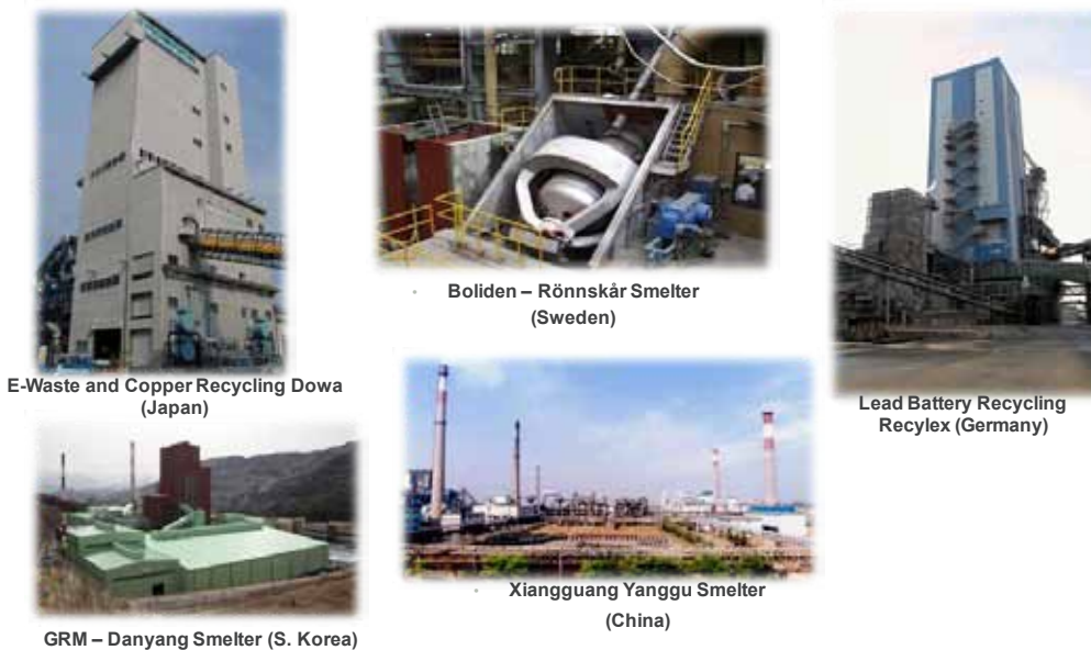
Figure 7. Versatile Outotec Smelting Technology accepting a range of feed types including copper, lead, various scrap, residues and eWaste (two left plants) .
