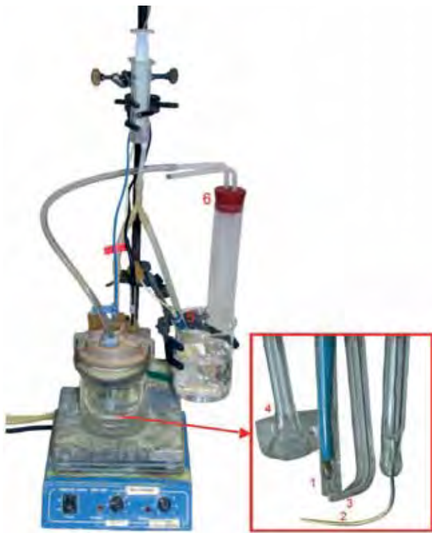
Fig. 1. Experimental setup: 1 PGM-wire working electrode, 2 Pt-counter electrode, 3 Capillary tip, 4 Gas purging, 5 Reference electrode, 6 Water lock.
