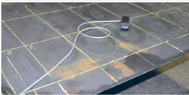
An 8 mm unannealed EHS-Steel plate together with the probe for the MikroMach.
