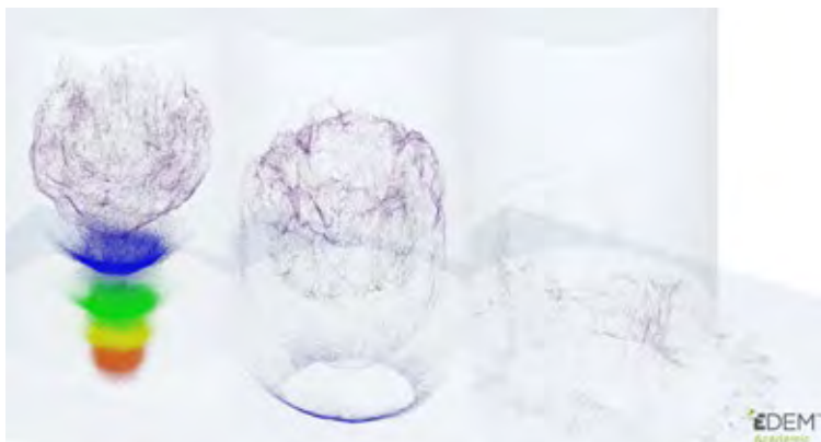
Figure 4. An example of simulation results with EDEM (coupled CFD-DEM) presenting a sequence of different size particles descending through the reaction shaft of a flash smelting furnace (isothermal, non-reactive case).
