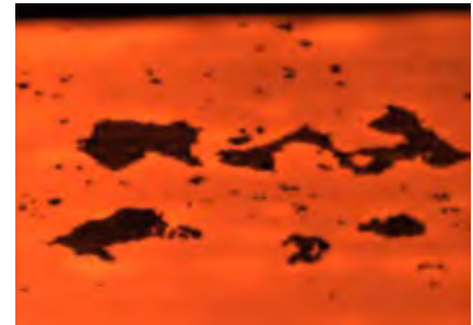
a) After pass 1: Discharge temp 1140°C. The residual scale was hot rolled in one pass
