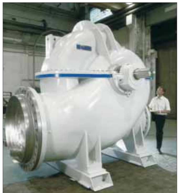
Figure 5. Biggest feed pump (breast box) of the world produced by Sulzer Pumps Oy Karhula Foundry.
