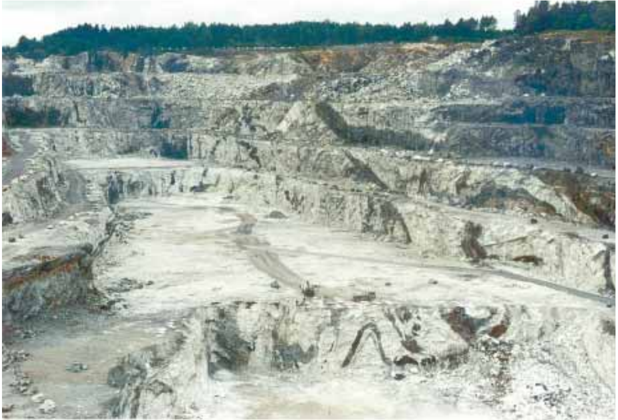
The folded and inhomogenous character of the Pargas limestone requires strict quality control and a selective mining system.
