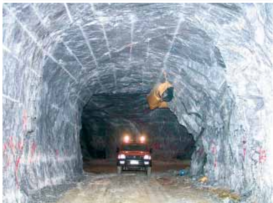
Development drift at Orivesi gold mine.
