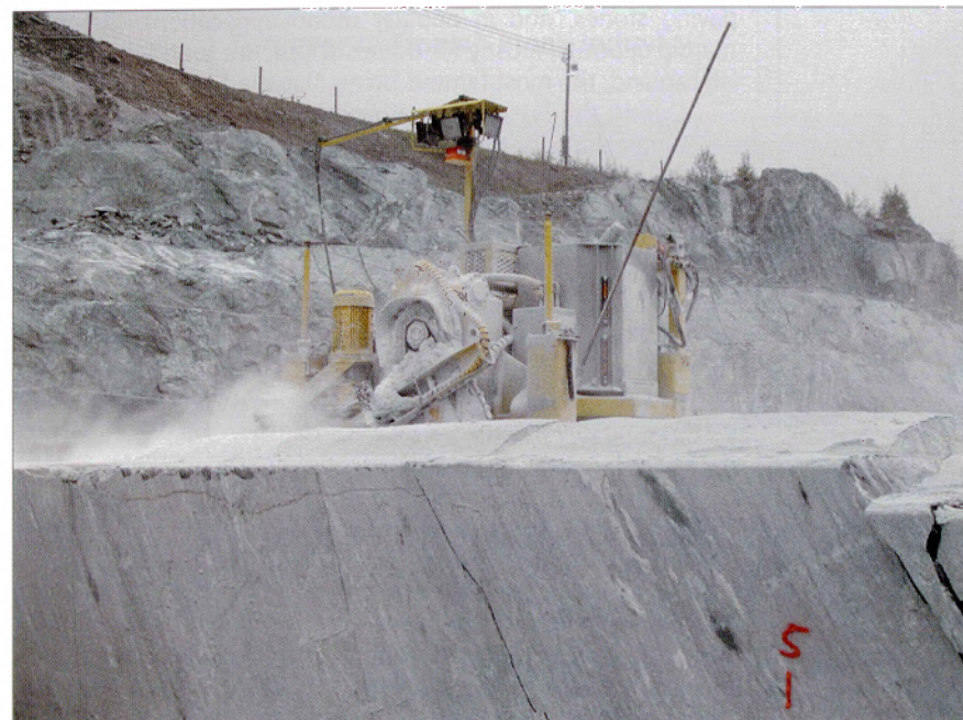
Figure 3. Vertical sawing of soapstone in Juuka. Soapstone is quarried with chain saws, operating both vertically and horizontally. The sawing loosens a ledge from which the soapstone blocks are removed with a wheel loader. Photo: Paavo Härämä.
