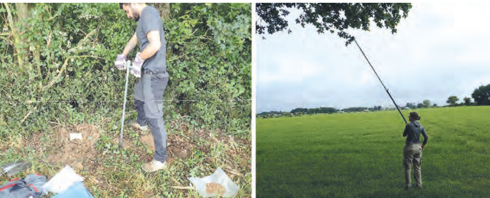
Figure 4. Soil sampling using a hand auger (on the left) and oak twigs (on the right) in the Vendée antimony district, France.
