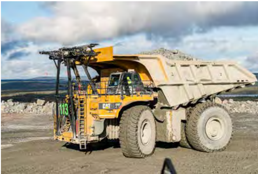
Figure 4: Trolley modified Cat 795F AC in Aitik
