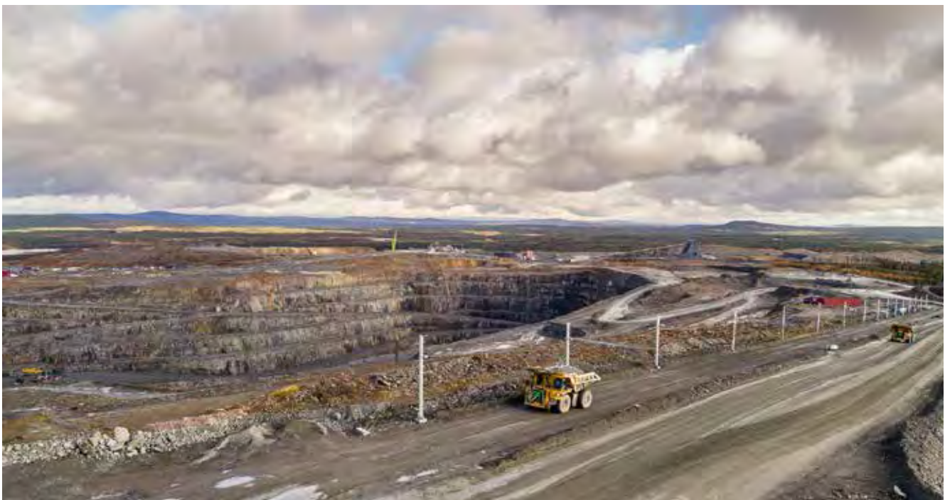
Figure 5: Trolley lane in Aitik mine leading up to the waste dump. Main pit is in the background.
