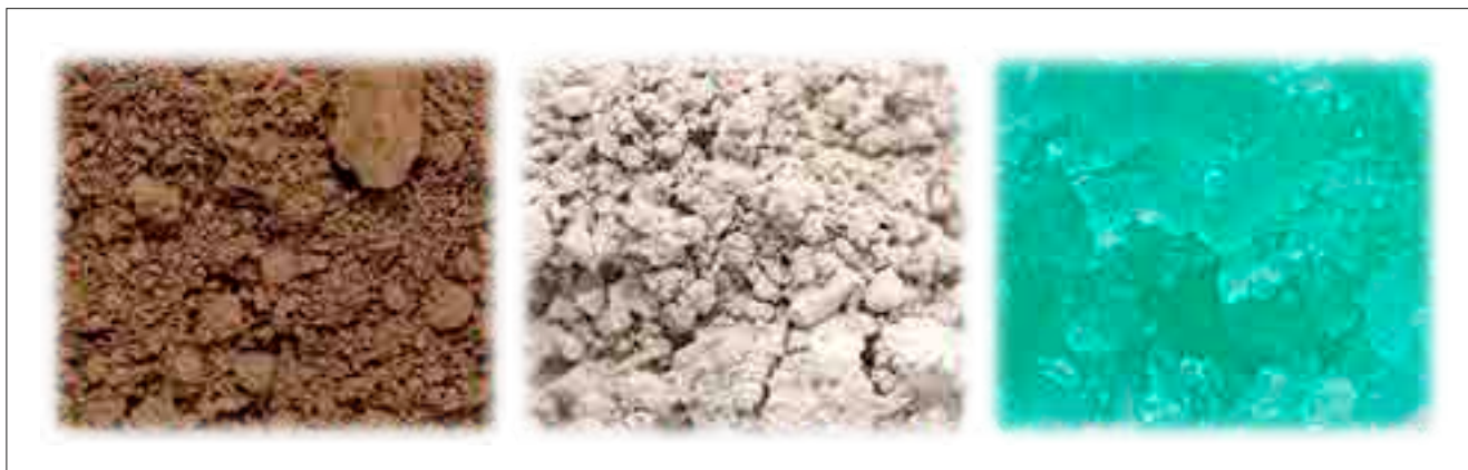
Figure 2. EAF dust (left) with the two main products Zn-sulphide and Fe-sulphate_heptahydrate
