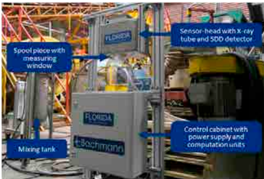
Figure 2. FLORIDA XRF analyzer during the test campaign at GTK Mintec plant.
